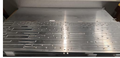
Fig. 2. Aluminium cold plates for the advanced thermal absorber
