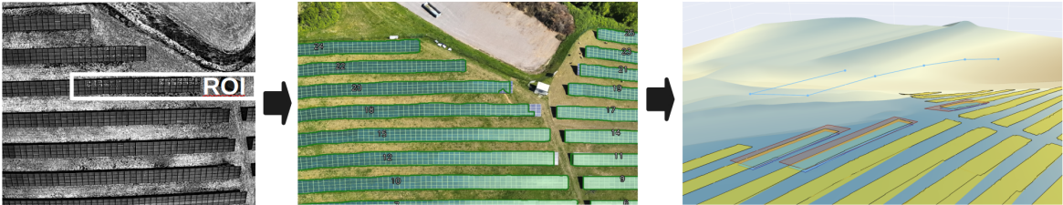
Fig. 2: Region-of-interest generation from overview IR imagery and anomaly detection, RGB module area detection projected onto the terrain model, 3D modelling with optimal flight path generation
