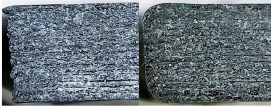
**Figure 2.** Comparison of the partial cross-sections of two specimens-x before (left) and after (right) being treated with acetone vapour during 30 minutes.
