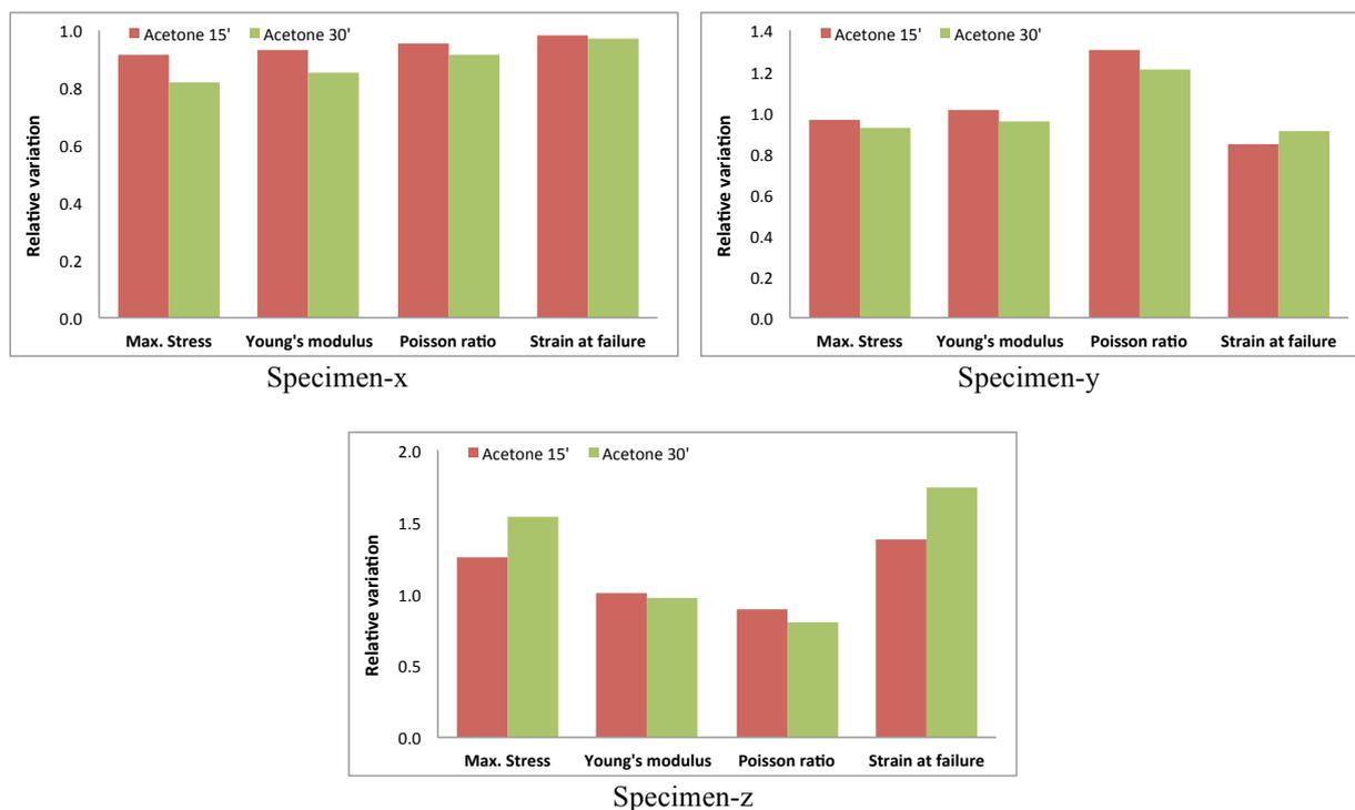
**Figure 5.** Relative variation of the maximum stress, Young's modulus, Poisson ratio and strain at failure with respect to the values of the non-treated specimens for the three specimen configurations.
