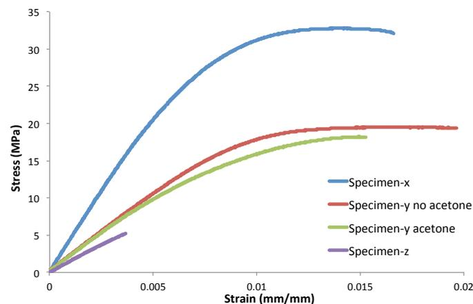
**Figure 3.** Representative stress-strain curves for the three specimen types (for specimens-x and -z the curves are similar with and without acetone vapour while for specimens-y the response varies if they are treated with acetone vapour or not).
