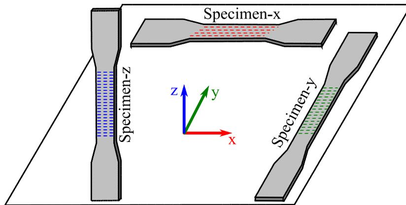
**Figure 1.** Schematic representation of the three characteristic directions considered for printing the specimens (the dashed colour lines in the specimens represent the orientation of the filament).
