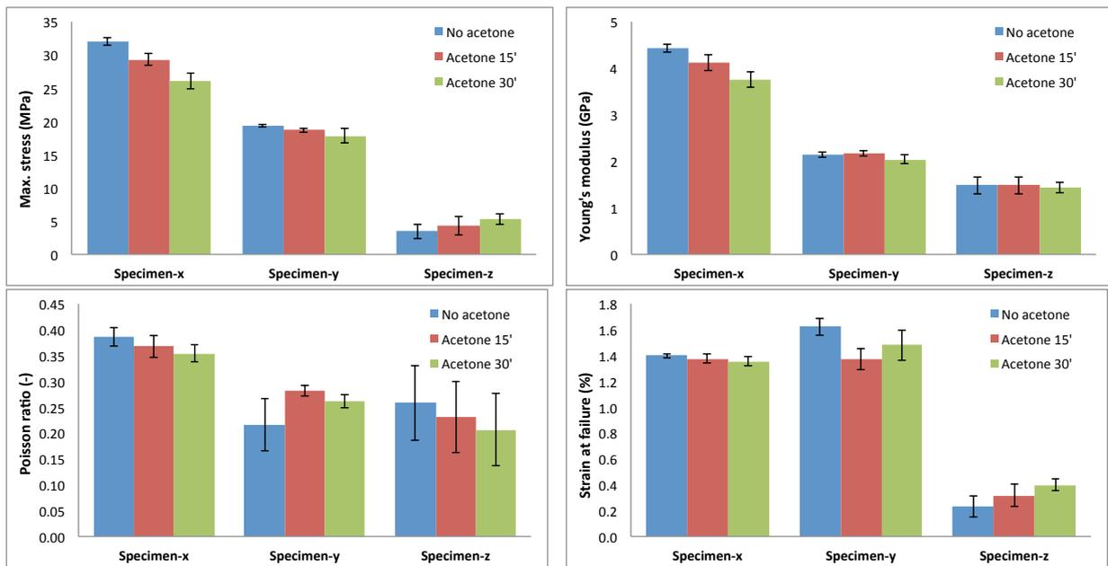
**Figure 4.** Average values of the maximum stress, Young's modulus, Poisson ratio and strain at failure for the 45 coupons tested under tensile loading.
