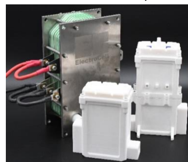
Size comparison of COTS electrolyzer versus LANL-developed electrochemical flow cell. Two versions of bespoke flow cell are shown with the short cell in front, and the tall cell in back.
