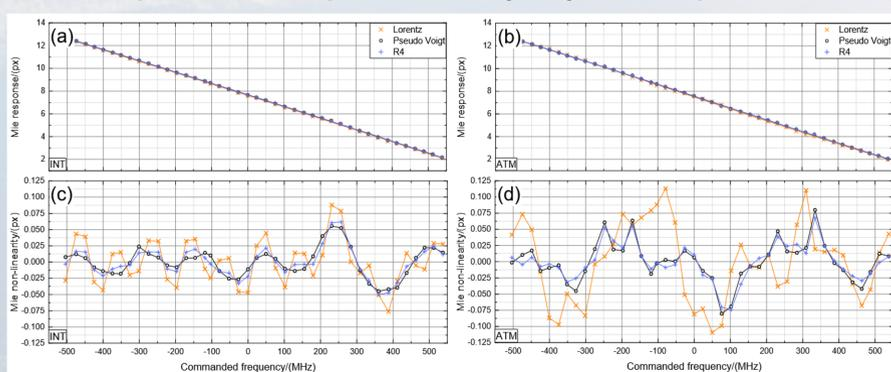
Fig. 4: Mie response of the internal reference signal (a) and ground return signal (b) retrieved by the Lorentzian fit (orange), the pseudo-Voigt fit (black), and the  $R_4$  algorithm (blue), from data acquired with the A2D on 18 September 2019 (AVATAR-I). The residual to a third-order polynomial fit is shown below in panels (c) and (d).
