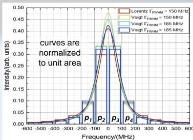
Fig. 2: Fizeau fringe profiles simulated by different model functions (Lorentzian and pseudo-Voigt) and different widths (see label) for a spectral pixel width of 100 MHz (bars).
