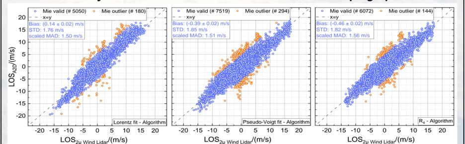
Fig. 5: A2D Mie cloudy LOS winds plotted against the 2- $\mu$ m DWL wind speed projected onto the A2D LOS direction for the 10 research flights performed during AVATAR-I, analyzed with the Lorentzian fit algorithm (left), the pseudo-Voigt fit algorithm (middle) and the  $R_4$  algorithm (right). Valid wind measurements are indicated in blue, and outliers that exceeded a modified Z-score threshold of 3.5 are indicated in orange, respectively.
