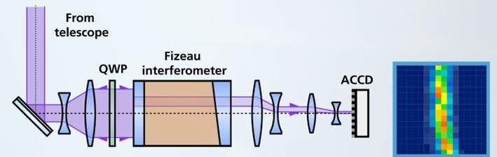
Fig. 1: Simplified sketch of the A2D Mie channel setup. QWP: quarter wave plate, ACCD: accumulation charge-coupled device.
