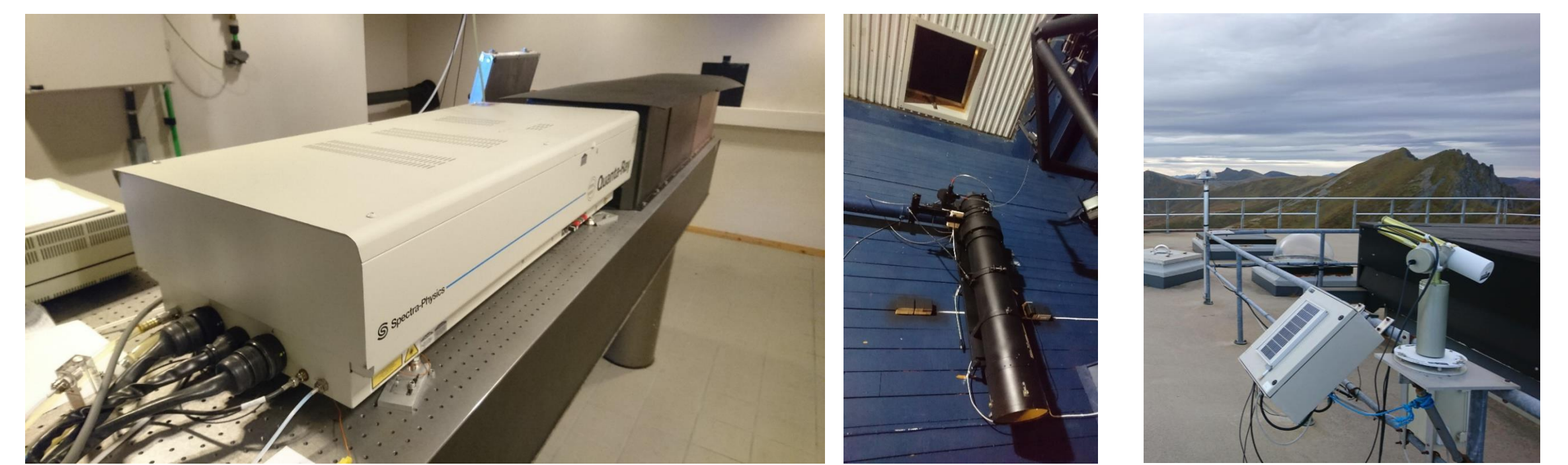
(Left) The ATL laser generator and (Right) the ATL beam guiding mirrors and receiver telescope.
