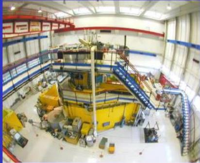
Thermal pool reactor, based on the TRIGA MARK II design by General Atomic.
