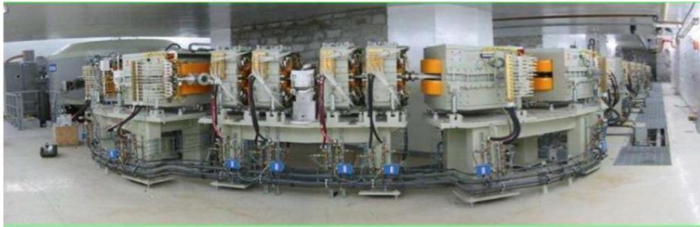
ESS = proton degrader + 'beam analyzer'
