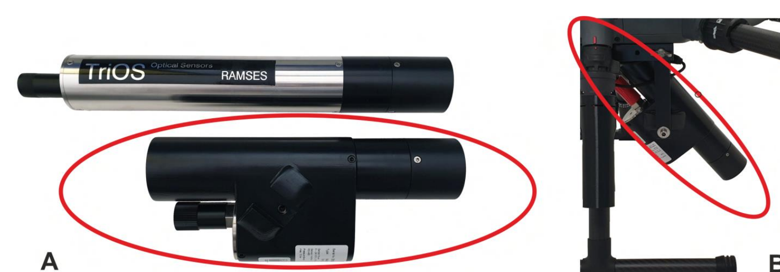
(A) L_T radiometer in the original steel case and that refitted in the new one (the encircled unit). (B) L_T radiometer deployed underneath the drone (the encircled component).
