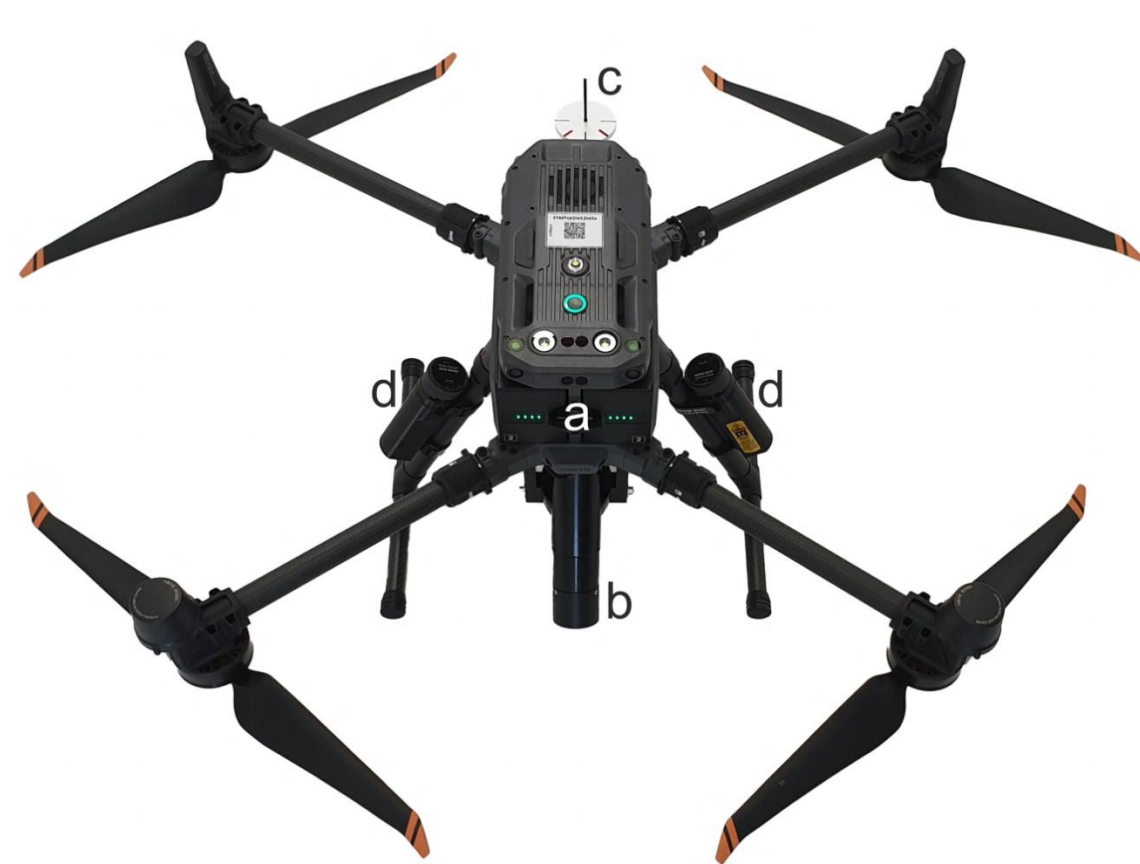
HYDRA: (a) Matrice 350 RTK; (b) L_T radiometer; (c) sun-alignment jig; (d) inflatable buoys.
