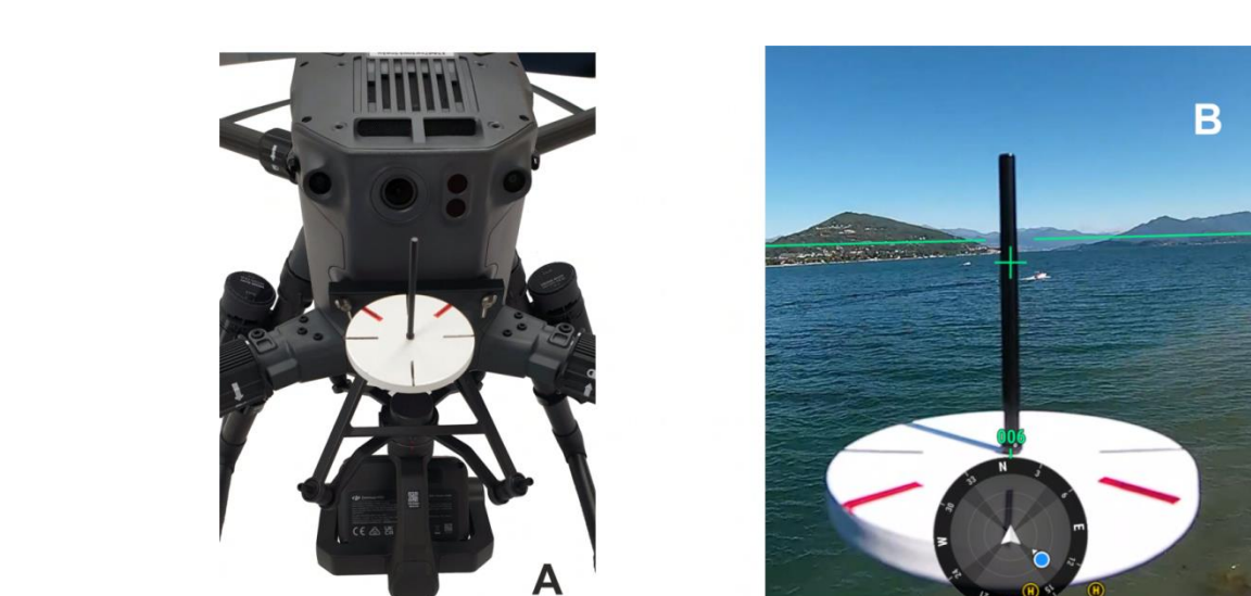
(A) sun-alignment jig installed in front of the fixed camera of the drone. (B) alignment jig as seen through the drone camera with the spike shadow indicating approximately \phi = 45^\circ with respect to the sun azimuth
