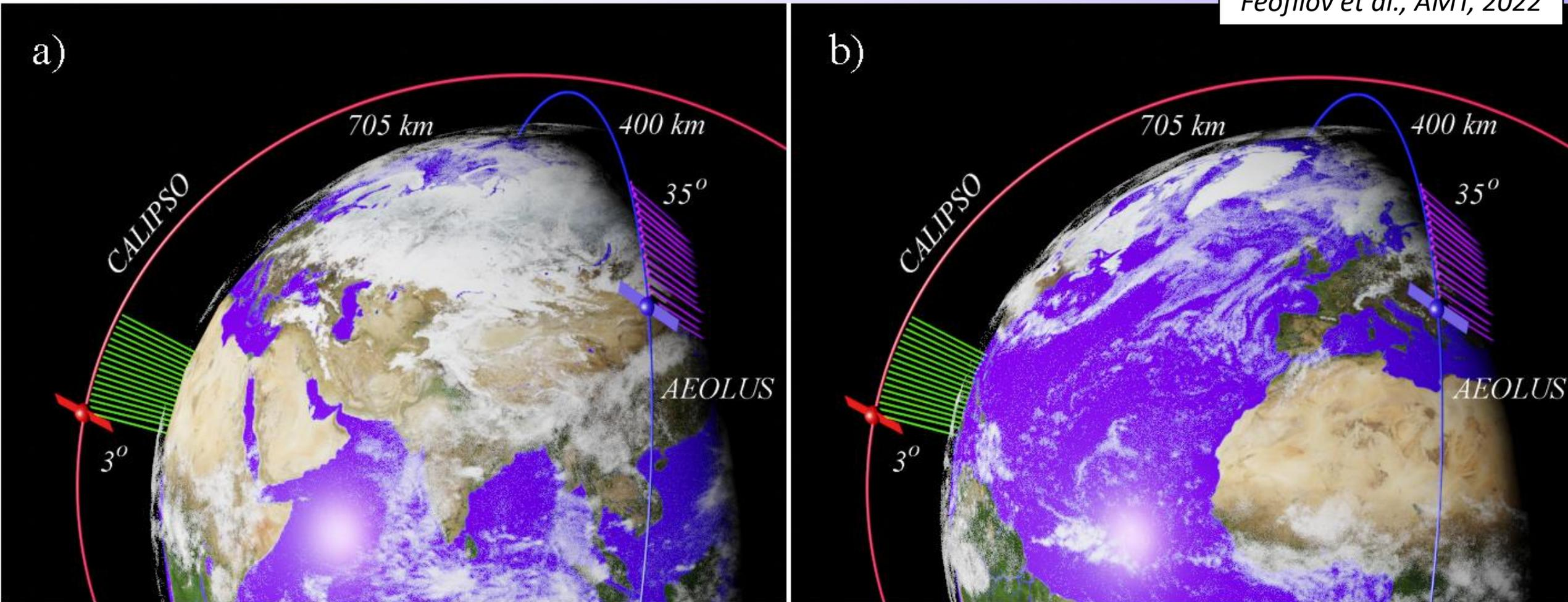
Observation geometry and orbits of ALADIN/Aeolus and CALIOP/CALIPSO space borne lidars. ALADIN observes the atmosphere at dawn-dusk, whereas CALIOP passes the equator at 01:30 and 13:30 local solar time. The difference between (a) and (b) panels is in the position of Earth and the time: in (b), AEOLUS overflies the same area (centered over Africa) as was observed by CALIOP ~4.5 h earlier (in (a)).
