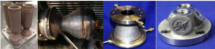
NASA MSFC rocket **injectors** made by AM resulting in a 70% reduction in cost.
