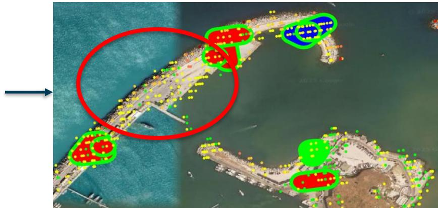
Isolated PS/DS, i.e., measurement points that do not fall within the clusters of anomalies: PS/DS that do not generate spatial/spatio-temporal anomalies. It is planned to use the displacement time series obtained along the LOS (Line of Sight) and extracted from the EGMS geoportal
