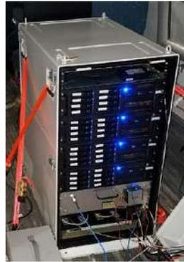
Ultrawideband microwave radiometer to image ice sheet internal temperature (e.g. Yardim et al. 2021)
