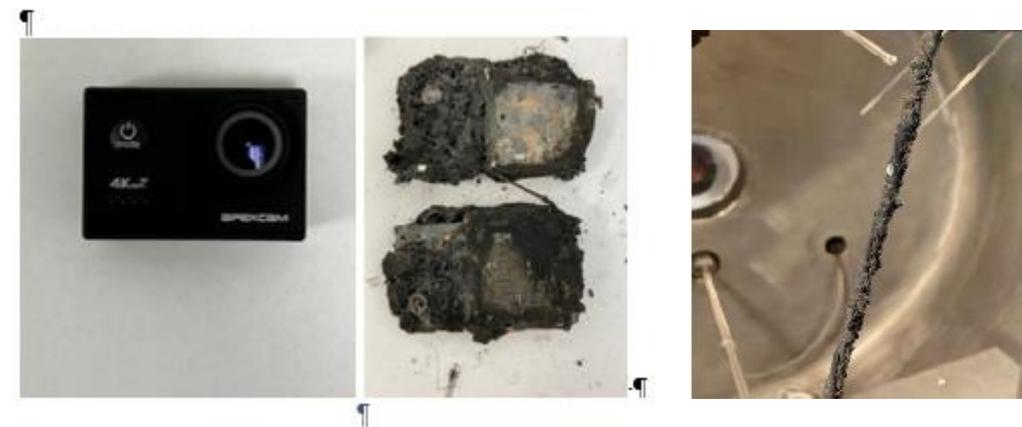
Configurational test : Action camera pre (L) and after test (R)
