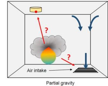
Modeling has shown that in zero-g with forced convection, the spacecraft volume must reach the alarm level before an alarm will sound:
