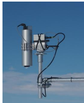
HYPSTAR® system [https://hypstar.eu/] 380-1700nm, 3-10nm FWHM
