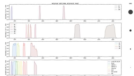
Figure 10. Relative spectral response of PlanetScope SuperDoves (bottom row) and Sentinel-2 bands at 10 m, 20 m, and 60 m GSD.
