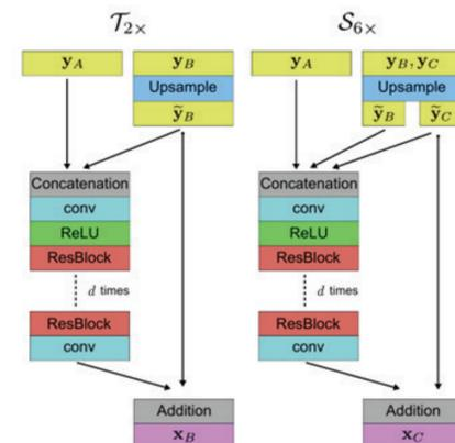
Figure 5. Architecture for DSen2 and VDSen2 proposed by Lanaras et al. 2018. Figure taken from the paper.
