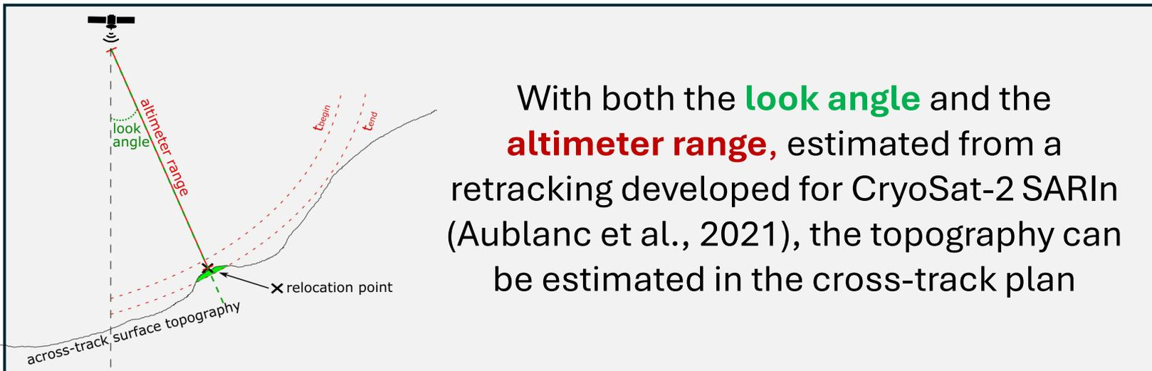
With both the **look angle** and the **altimeter range**, estimated from a retracking developed for CryoSat-2 SARIn (Aublanc et al., 2021), the topography can be estimated in the cross-track plan
