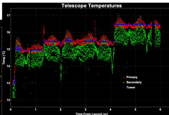
The setpoint for the telescope tower temperature has been adjusted during the mission to maintain control authority, preventing undesirable gradients.
