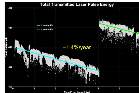
After two years at Level 5, the slope of laser pulse energy appears nearly identical to the slope observed at Level 4.
