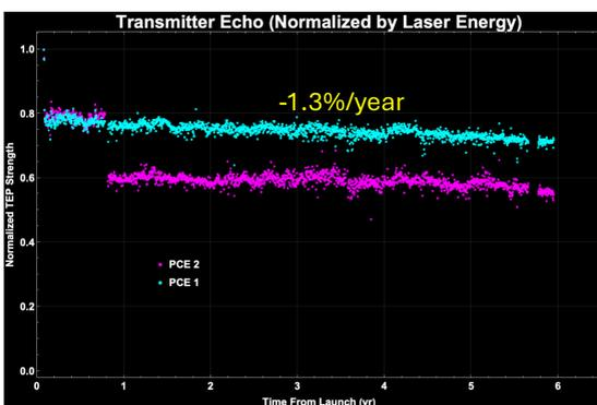
Strength of the two Transmitter Echo pulses per unit of transmitted laser energy
