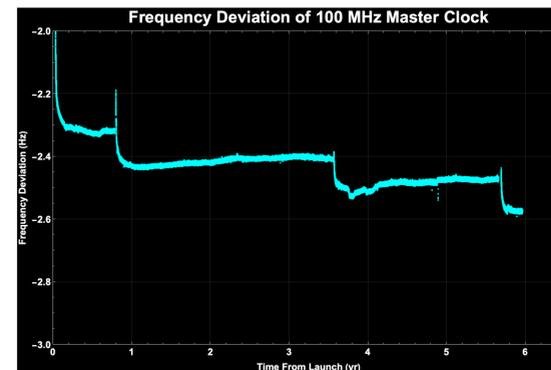
Each time the instrument has been power-cycled, the clock frequency has stabilized at a different value.
