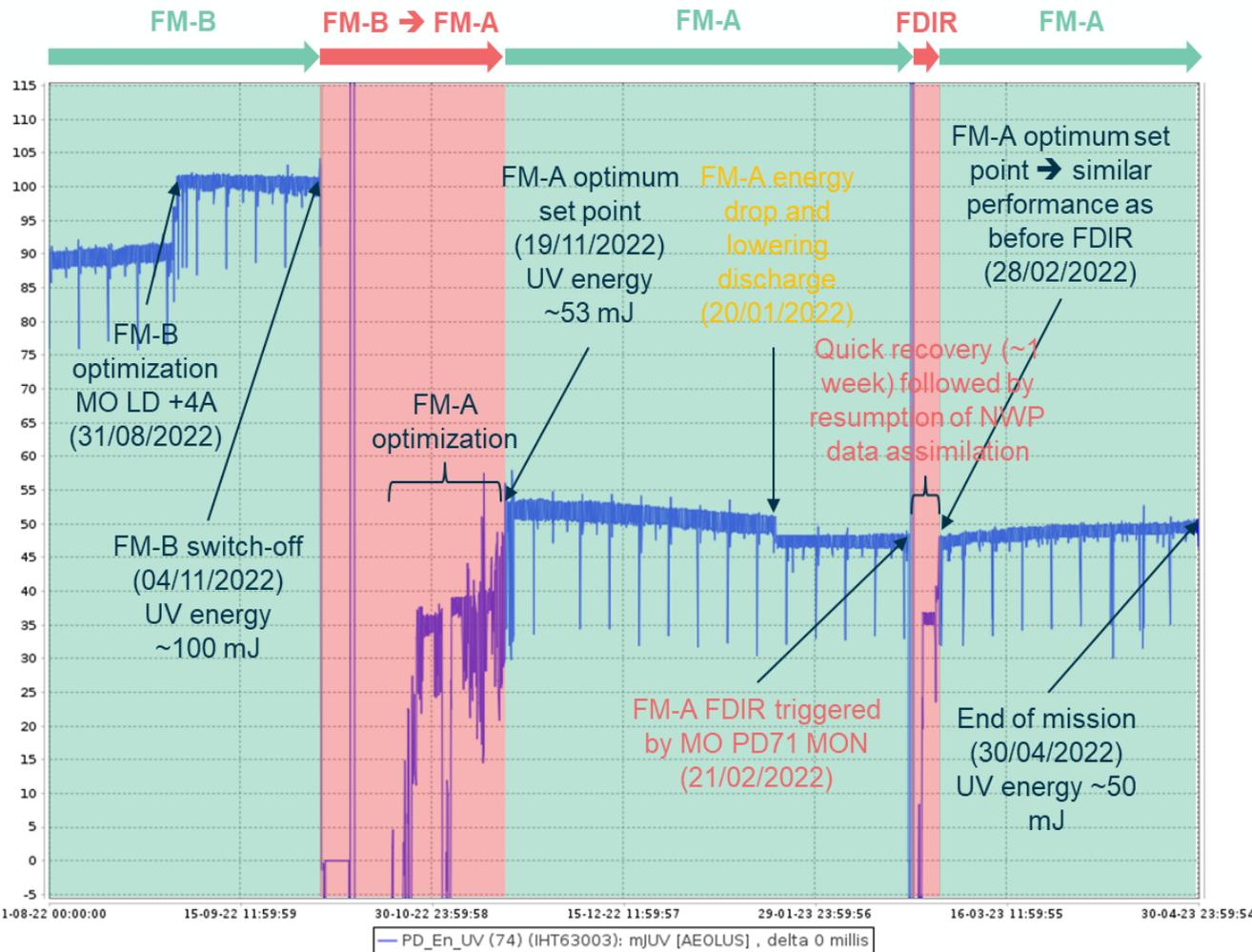
Laser UV output energy from the end of FM-B, switch-back to FM-A with main events towards the end of the operational mission lifetime.
