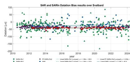
Fully Focused (FF) analysis exhibits a drift of approximately 0  $\mu$ s/year. Conversely, the stack analysis reveals a slightly higher drift, approximately 1  $\mu$ s/year.
