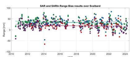
In Svalbard, the correction of the terrain motion was added to the other geophysical corrections to get the proper deviation of the instrument range bias. Resulting in a drift of less than 1 mm/year.
