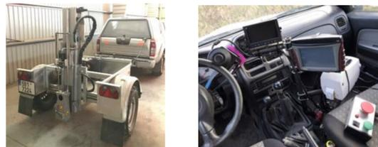
Semi-automatic sampling machine Niefeld N2006 used for soil sampling at farm Rostenice a.s.
