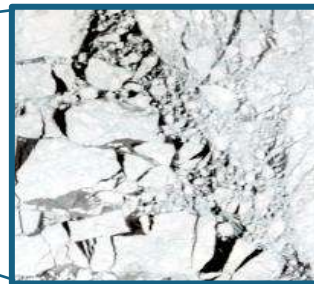
Extracted 100 × 100 pixel georeferenced "clean" tile centered on a valid SRAL measurement location
