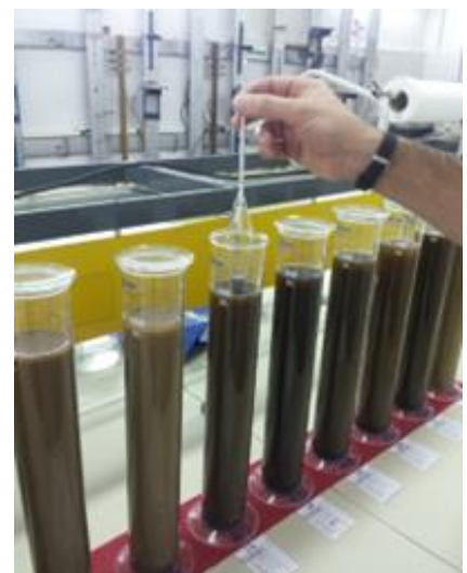
Grain size analysis Hydrometer method % of sand silt and clay
