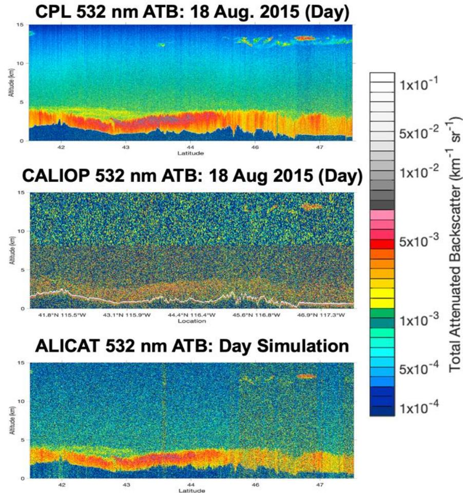
CPL data from the NASA ER-2 aircraft (top panel) and CALIOP (middle panel) during a validation flight on 18 August 2015 over the western US. ALICAT ATB (bottom) simulated for day using the airborne lidar data as input.
