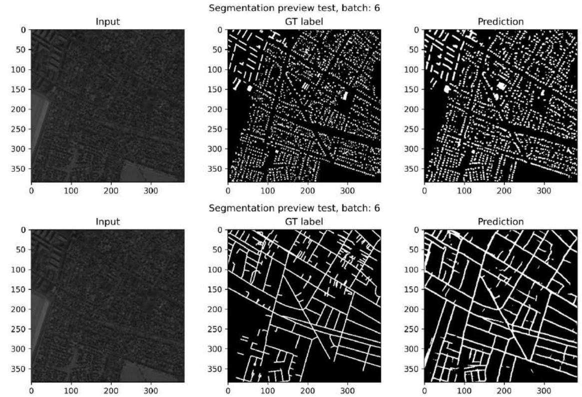
Figure 1: Exemplary segmentation networks results for buildings (top row) and roads (second row) obtained from the HR image from MuS2 dataset. The first column contains input images, the second the ground-truth (GT) segmentation masks (obtained via OSM) and the last one the predicted segmentation masks.
