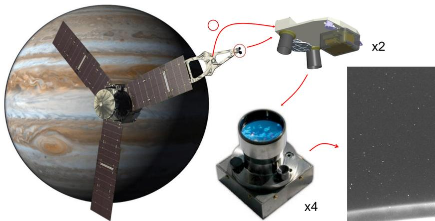
Figure 1: microASC cameras on the Juno MAG investigation optical benches. Image Credit NASA, DTU
