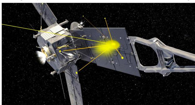
Figure 2: Spallation products from spacecraft dust impacts. Image credit NASA
