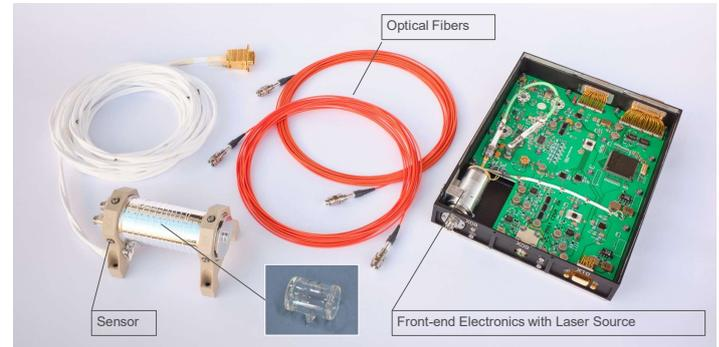
Flight model of the Coupled Dark State Magnetometer aboard Macao Science Satellite 1
