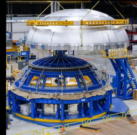
Artemis III Space Launch System Core Stage Liquid Oxygen Aft Dome
