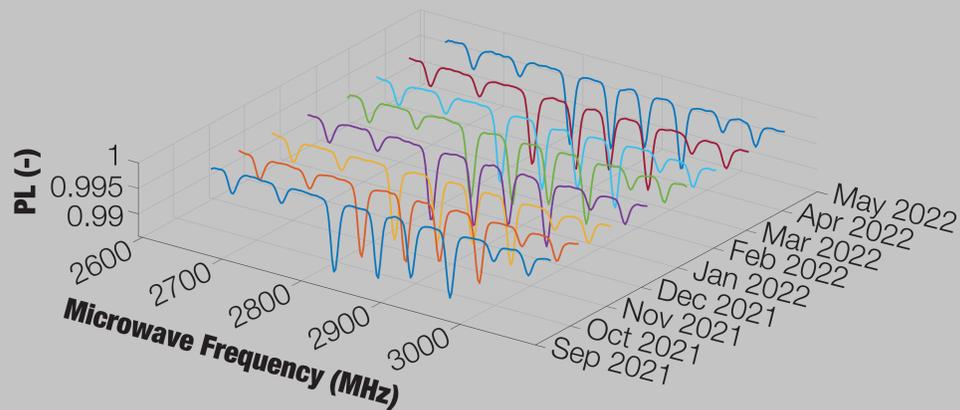
To assess the degradation of the OSCAR-QUBE sensor, measurements over a span of nine months were acquired. Normalized photoluminescence ODMR spectra with the eight peaks for comparison show no degradation, proving the feasibility of this technology in long-duration missions in space environment.
