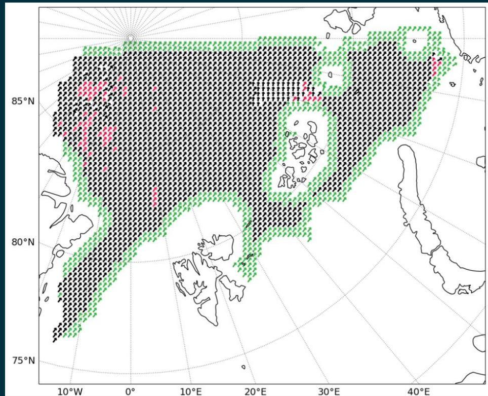
*Resulting motion vector field. The color encodes a status\_flag (green = close to land, ocean, or edge of the swath, red: corrected using neighboring vectors).*
