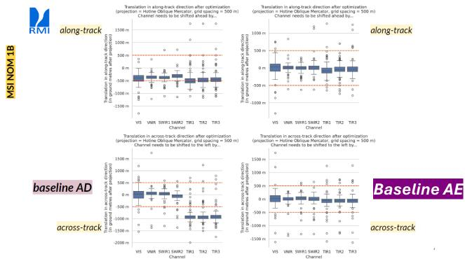
L1B Accuracy results showing compliance to requirements verified on "baseline AE" that is to say the last up to date release of image products set.
