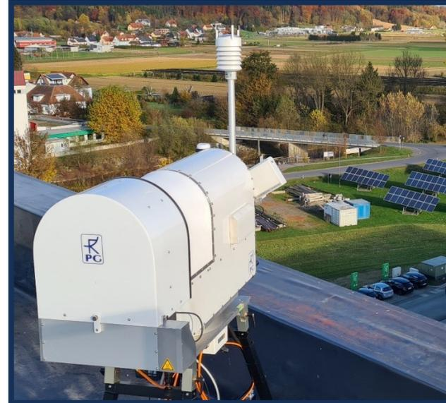
NubiScope **Infrared Cloud Structure Radiometer**
