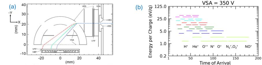
Figure 1: (a) schematic cross section of IRM sensor, showing simulated ion trajectories for  $V_{SA} = -174$  V at  $E/q = 1.3, 12.5$  and  $45.0$  eV/q (cf. Yau and Howarth 2016) and (b) time of arrival (TOA) ranges for various ion species at  $V_{SA} = -350$  V for the 6 lowest energy pixels
