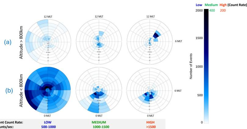
Figure 5: Occurrence distributions of molecular ions (a) above and (b) below 800km shown for events with high, medium, and low count rates. Observed distributions suggest more frequent occurrence of fast acceleration at low altitudes in the nightside auroral ionosphere compared with the dayside, and likely continuation of acceleration to higher altitudes in the dayside cleft.
