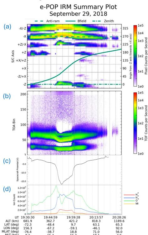
Figure 2: IRM summary plot showing (a) energy-time spectrograms at 8 angles and (b) time of flight spectrogram of measured ions, and (c) inferred spacecraft potential and (d) ion composition
