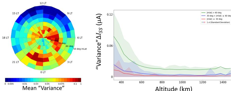
Figure 7: (a) Magnetic latitude-local time and (b) altitude distributions of 'variance'  $\Delta I_{SS}$  of measured sensor surface current  $I_{SS}$  as a proxy for  $\Delta n_e$
