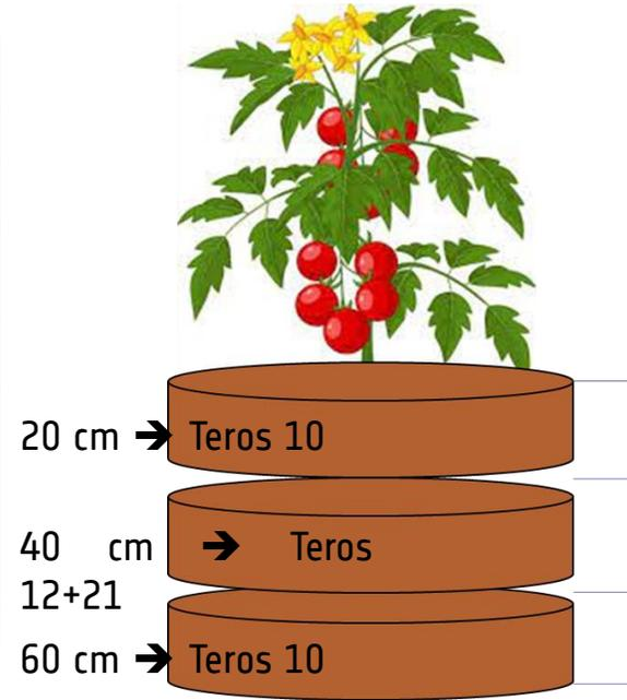
SM has been measured at a depth of 20, 40 and 60 cm with a sampling time of 15 min. In 2022, measurements were collected from May, 19 till Aug, 26.
