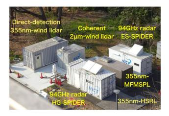
The high sensitivity doppler cloud radar (HG-SPIDER; -40dBZ at altitude of 15km) obtained consistent radar reflectivity and doppler velocity with CPR\_ECO.
