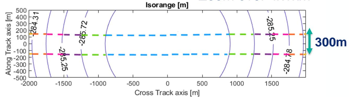
Different colors of dashed line represent different resolution cells at intervals of 47cm range delay
