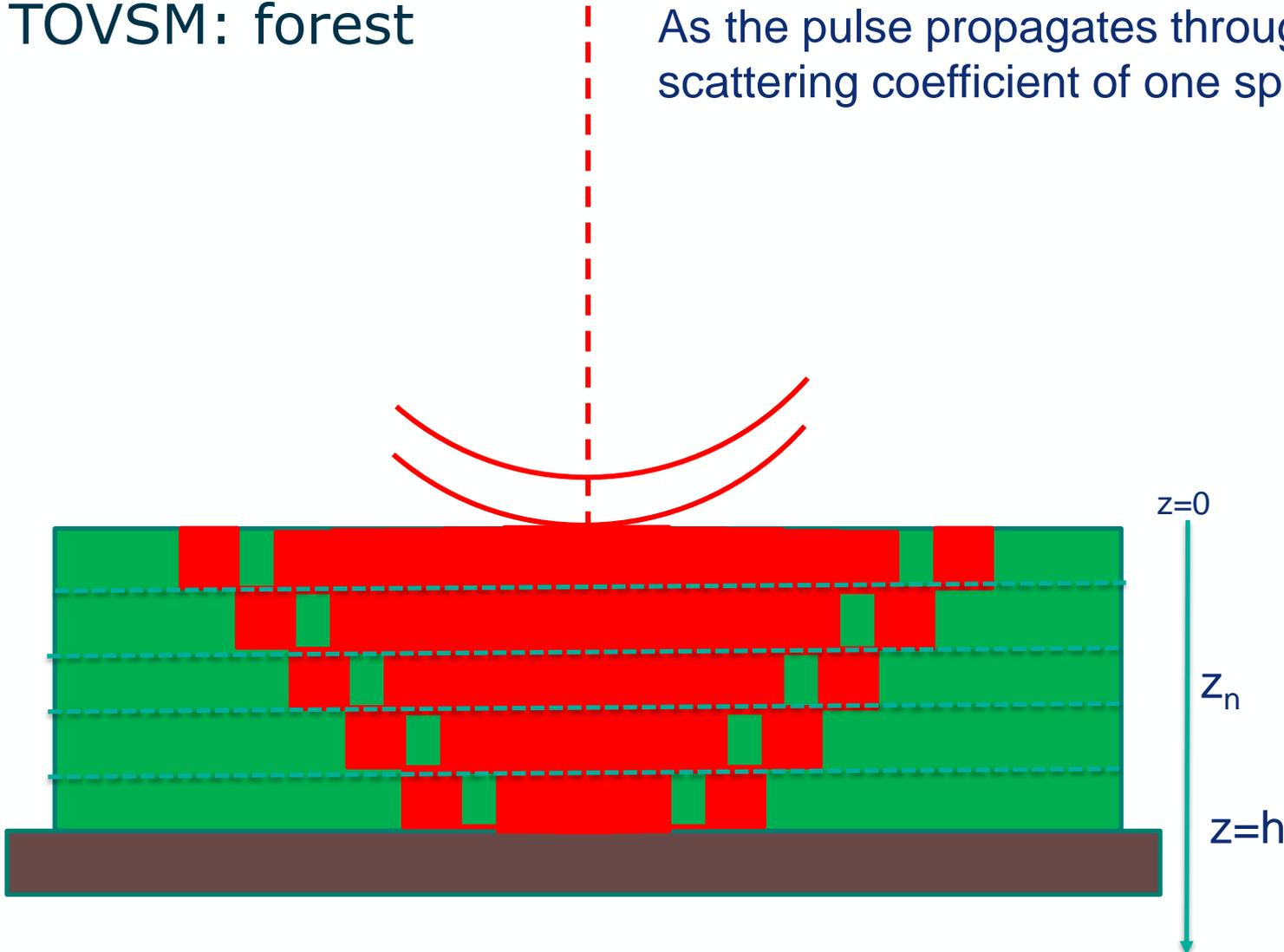
The incident and scattered power are attenuated by the above layers. Both **volume scattering** and **attenuation increase as the number of layers increases.**
