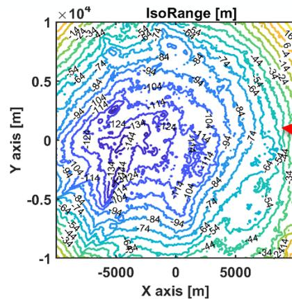
Concentric ring shapes of the iso-delay lines are distorted by the surface elevation
