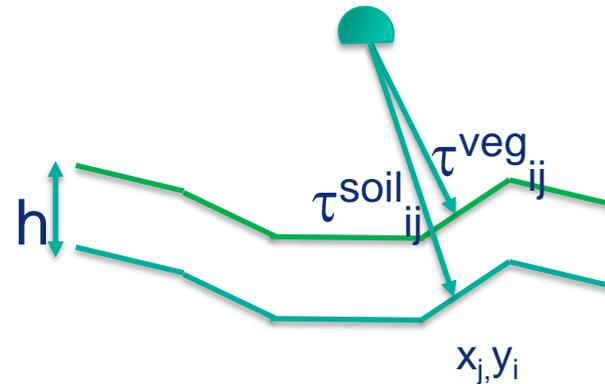
The contribution from element  $x_j, y_i$  will be included in the radar equation weighted by the Impulse function and coupled with
