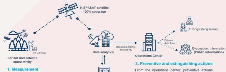
Sensors are deployed in protected areas and, thanks to the **satellite's ubiquity**, data is sent to the cloud-based data analytics system. 360° cameras are also considered and strategic points.
