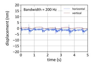
Unbeatable performance The attoDRY800xs offers excellent ultra-low vibration performance. The interferometric measurements measured directly on the cold plate show peak-to-peak vibrations in vertical direction are less than 2 nm (3 nm), while in lateral direction they are inferior to 10 nm (40 nm) in a bandwidth of 200 Hz (1500 Hz).
