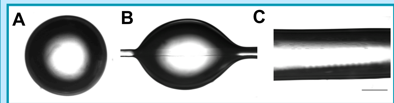
Figure 2. Representative brightfield images of hydrogel structures generated using a glass capillary microfluidic device. (A) Droplet, (B) interlinked bead, and (C) thread morphology. Scale bar = 500 μm.
