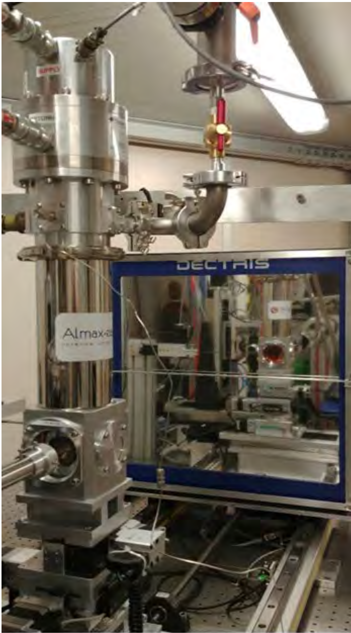
Figure 1. Closed cycle He-cryostat and PILATUS3 S 6M detector.
