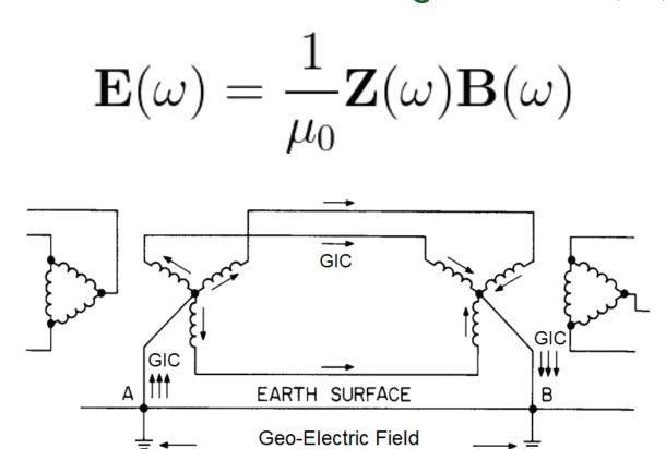
Schematic of GIC flow through high-voltage transmission line, up and down through the grounding points at the transformer neutrals [from Kappenman, 2010].
