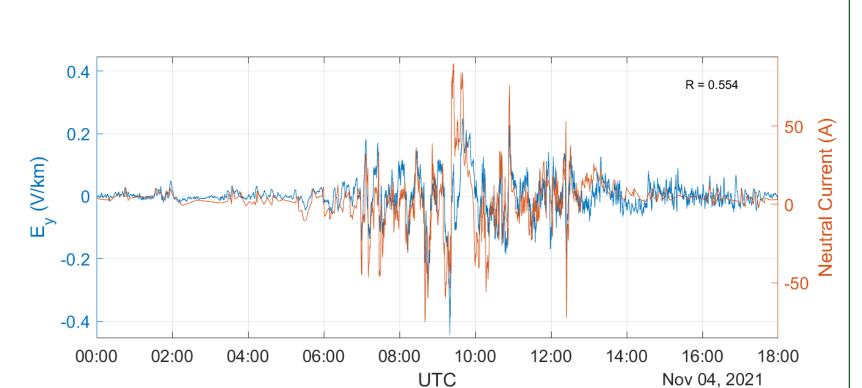
Local electric field derived using MT impedance and local GMD from MTSK station in the CARISMA array (blue). Measured transformer neutral to ground (TNG) GIC from Hall sensor (blue) (Parry et al., 2024).
