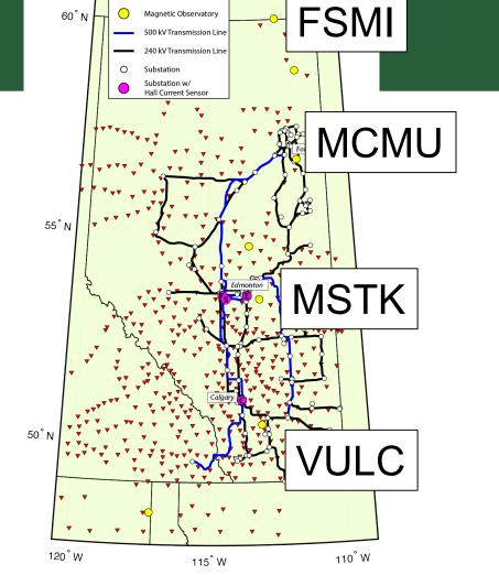
(left) CARISMA magnetometer array stations; (right) Map showing magnetotelluric (MT) and selected magnetometer stations, power network, and transformer neutral-ground Hall sensors in Alberta.
