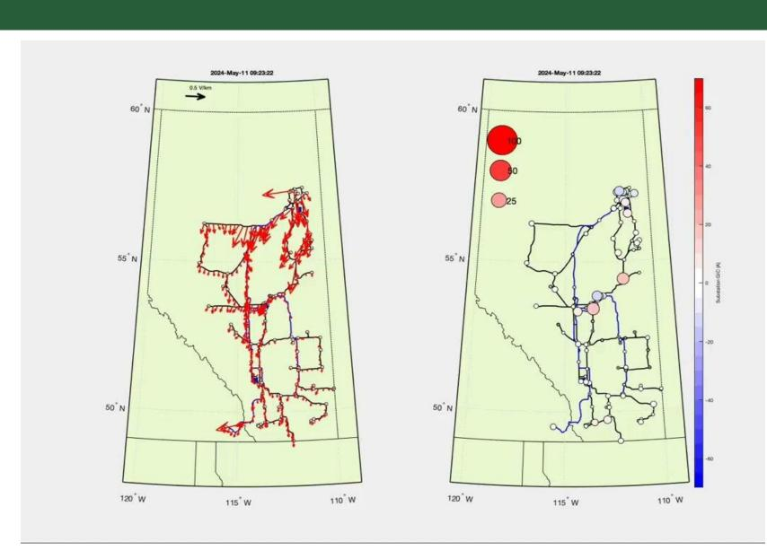
Combining E, determined from interpolated dB and MT impedance, and power network model characteristics allows a model to be used to assess GIC flows in the Alberta grid. Validated using Hall sensor TNG GIC sensor data.
