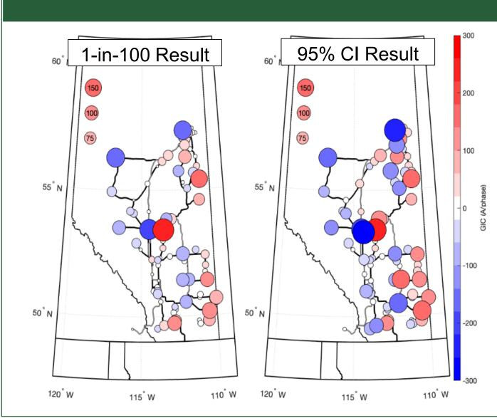
GIC model statistics for network driven by station-by-station extreme electric fields.
