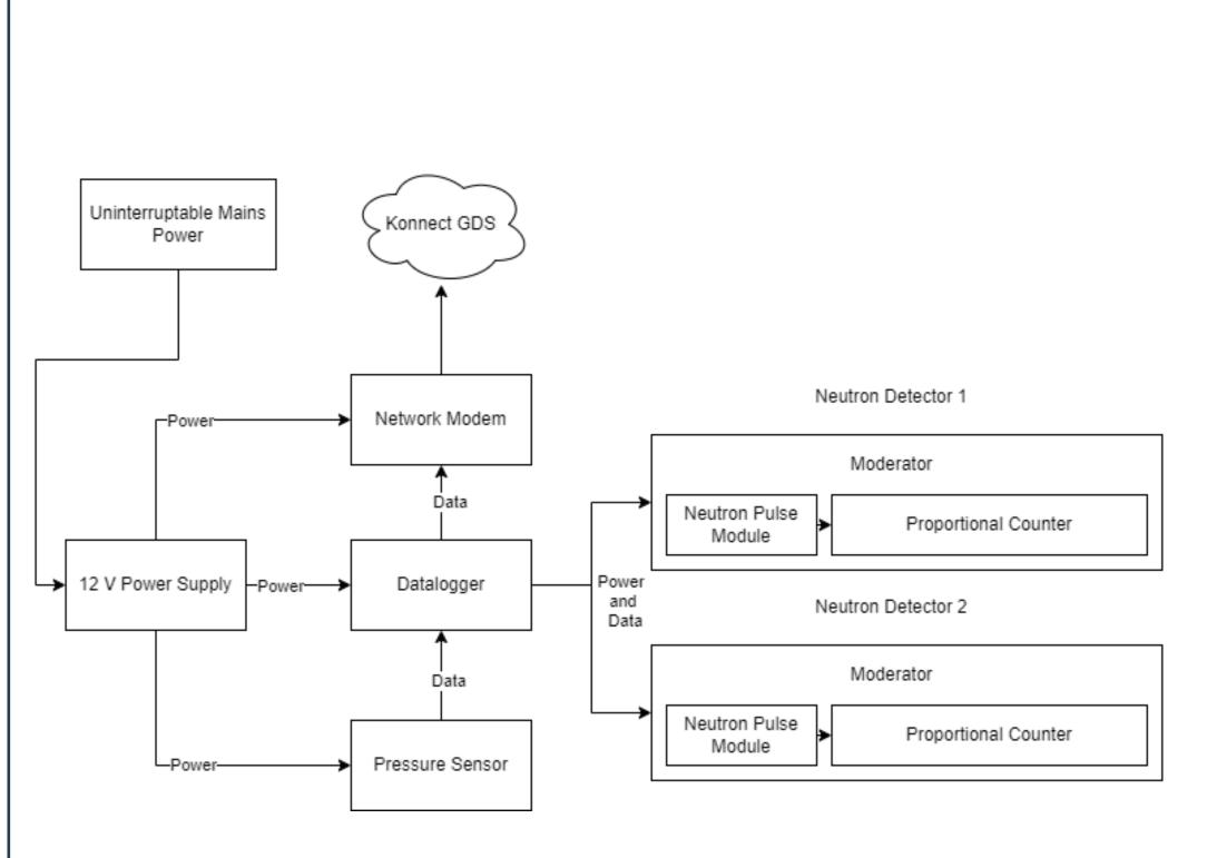
The installation consists of two moderated helium-3 neutron counters, with a pressure sensor for monitoring atmospheric pressure variations. The instrument is powered via a 12V power supply which is itself supplied by an uninterruptible power supply. Data is uploaded in real time to the cloud via a 4G mobile internet connection. The left image shows a block diagram of the instrument.
