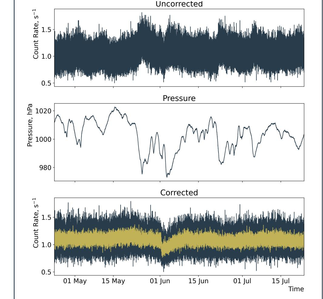
The **top panel** displays the total count rate of the CNM at 1 minute resolution, and the middle panel shows the measured atmospheric pressure at Lerwick. The bottom panel shows the result of correcting the data for pressure at 1 minute and 5 minute resolution (blue and gold respectively).
