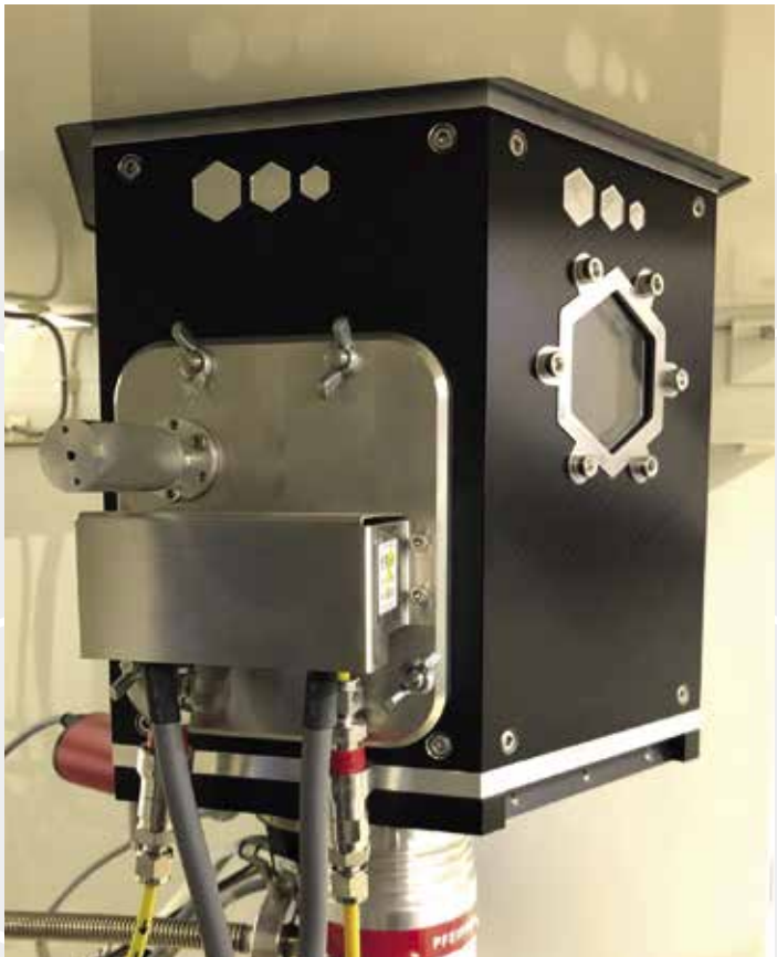
HEX-L on frame with electronics rack (Shown with optional load-lock mounted)
