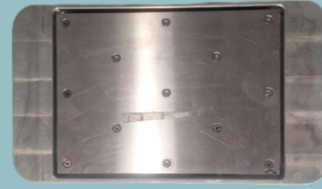
Custom nanovibration bioreactor, generating a 30 nm amplitude
