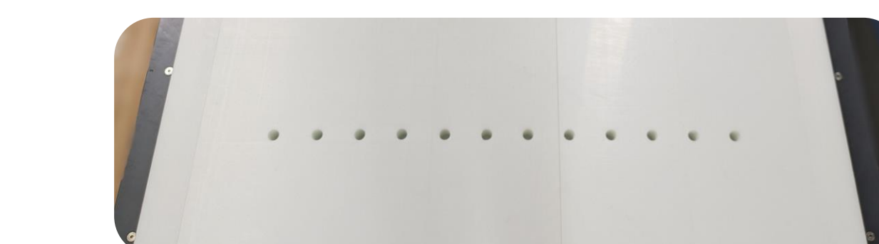
Figure 6: Measurement recesses in the top surface of the monitor
