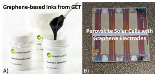
Figure 1 a) Graphene enriched carbon inks developed by GraphEnergyTech and b) Photograph of a PSCs with carbon-based electrodes.
