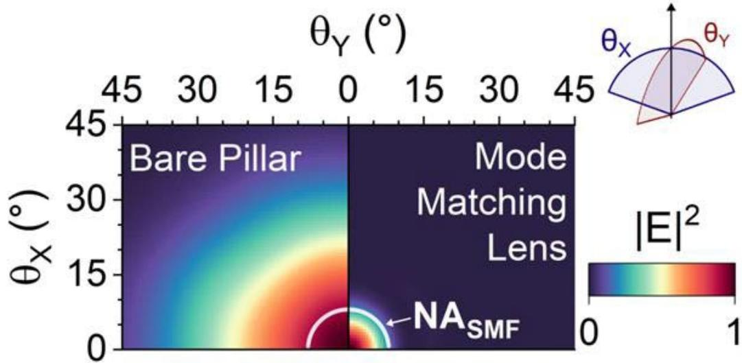
Fig. 1. The far-field profiles of the field intensity  $|E|^2$  are shown as a function of angle from the normal along the x and y axes ( $\theta_x, \theta_y$  as shown in the inset) for the lensless bare micropillar and the optimised  $R = 5.7 \mu\text{m}$ ,  $k = 0$ ,  $k_4 = 3.75 \times 10^{-3} \mu\text{m}^{-3}$  lens. The NA of a SMF is shown as a white circle.
