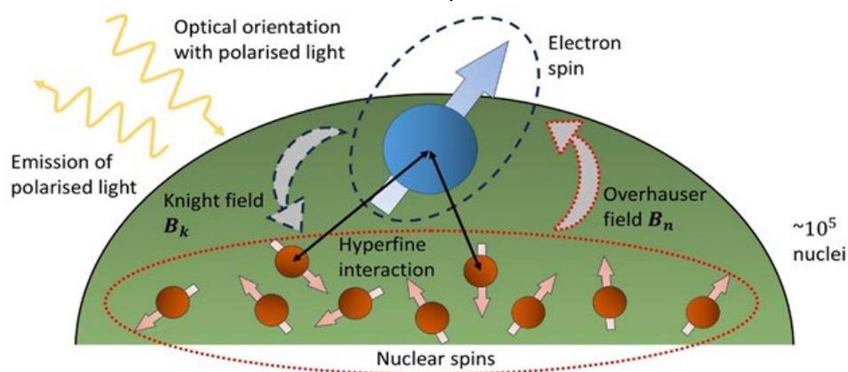
Figure 1: Diagram demonstrating the reciprocal interactions between electron and nuclear spins in quantum dots.
