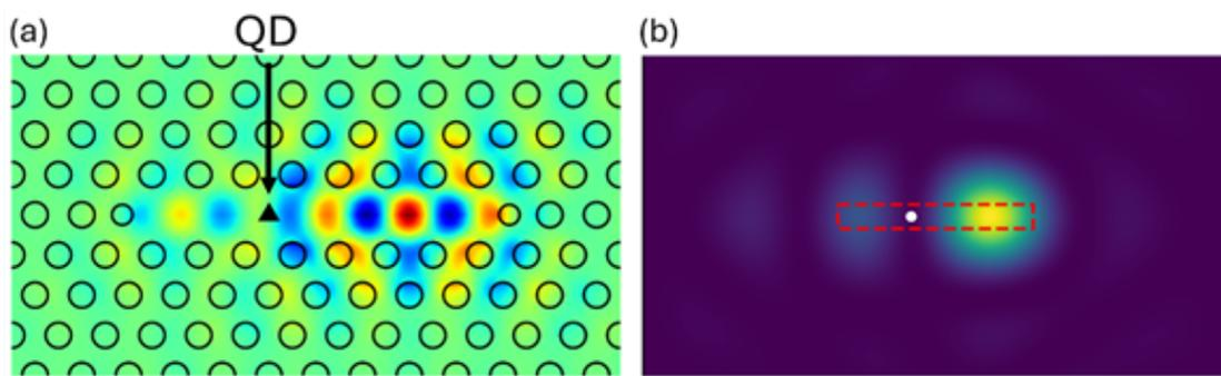
**Fig. 1:** (a) The intensity profile of the field emitted by a QD into the cavity. (b) The far-field image of the cavity formed by the emitted light at a different detuning; the locations of the QD and the cavity are marked with the white dot and the dashed line, respectively.
