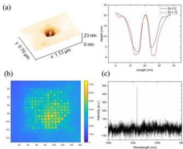
**Figure 1:** (a) A 3D of a single nanohole with one dot inside and its profile line (b)  $\mu$ PL image of the site-controlled QD area at 4 K. (c) Low temperature ( $T = 4$  K)  $\mu$ PL spectrum of an individual QD under low excitation power (1  $\mu$ W)
