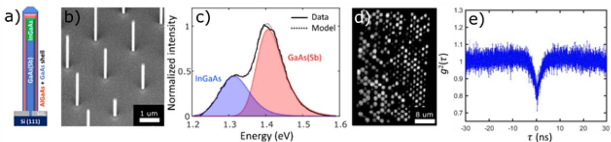
**Figure 1.**(a) Schematic of nanowire structures, (b) SEM image of nanowires, (c) 300K PL spectrum of one nanowire, (d) 5K single photon map of 400 QDs, (e)  $g^2$  measurement of one QD.
