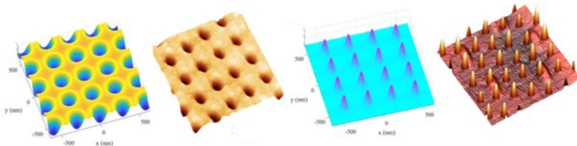
Simulated interference patterns and the resulting surface structures. Left shows the formation of nanoholes and right shows the accumulation of islands to form quantum dots
