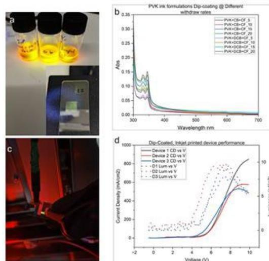
Fig: (a) InP QDs ink formulation (inset: QDs printed on glass with 40  $\mu\text{m}$  drop spacing); (b) absorption spectrum of the PVK film; (c) A electroluminescent QLED under turn on condition; (d) performance metrics of the fabricated devices.
