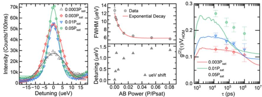
Figure 1: a) QD linewidth measured under resonance fluorescence with increased application of above-band excitation power expressed as a function of saturation power  $P_{sat}$ . b) QD linewidth and detuning as a function of above-band excitation power. c)  $g^{(2)}(t)$  measurements at different above-band excitation powers overlaid with HOM visibility measurements under the same conditions
