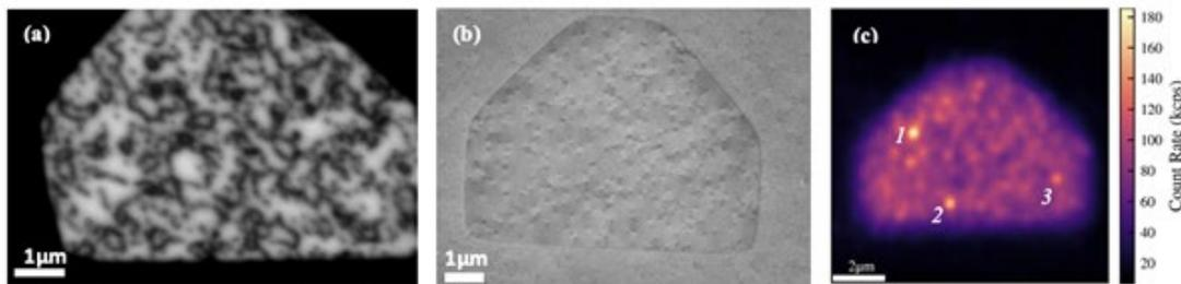
Fig 1. The same marked region of GaN on sapphire (a) Cathodoluminescence (CL) (b) Electron Channelling Contrast Imaging (ECCI) and (c) Photoluminescence showing bright regions of potential SPE.
