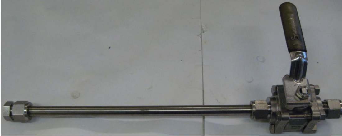
316 SS cylinder equipped with Swagelok valve
