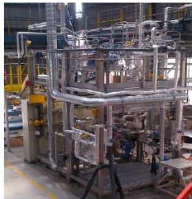
DMX™ Mini-pilot unit IFPEN, Solaize 0.5 kg/h CO 2 capture
