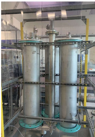
Figure 1. DAC Absorber and water wash columns used in this study.
