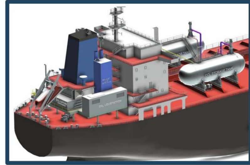
Figure 4. Conditioning and Capture equipment locations for 1 ton per hour capacity.
